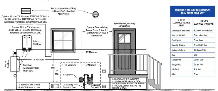
The preferred meter assembly location shall be at the front corner, along the front wall of the structure, or within 3 to 5 feet along either side wall from the front of the structure. On the garage side, the meter location shall be on the front side wall.
